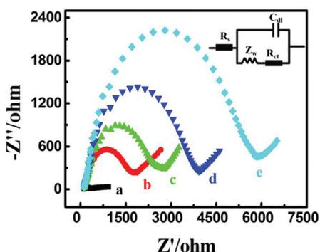
Fig. 2 EIS characterization of the different electrodes in 0.1 M KCl containing 5 mM  $[\text{Fe}(\text{CN})_6]^{3-/4-}$ : (a) bare Au electrode, (b) Fc-H1/Au electrode, (c) MCH/Fc-H1/Au electrode, (d) probe STP/MCH/Fc-H1/Au electrode, (e) MB-H2/probe STP/MCH/Fc-H1/Au electrode.
