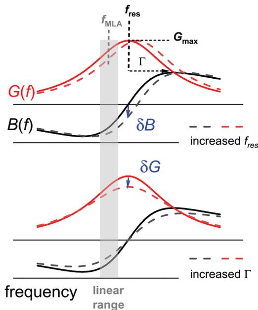
Fig. 2 If the only variable parameters of a resonance curve are the resonance frequency,  $f_{\text{res}}$ , and the half bandwidth,  $\Gamma$ , there is a one-to-one correspondence between the complex electric admittance  $Y = G_{\text{el}} + iB_{\text{el}}$  at one fixed frequency  $f_{\text{MLA}}$  (close to the centre of the resonance), on the one hand, and  $f_{\text{res}}$  and  $\Gamma$ , on the other.
