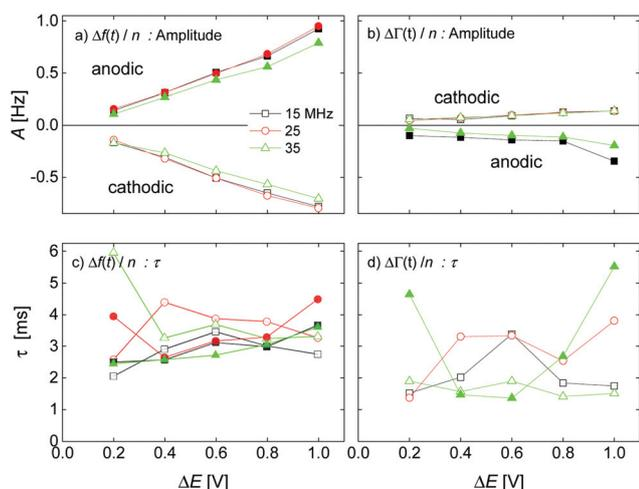
**Fig. 6** Dependence of amplitude  $A$  and response time  $\tau$  on the magnitude of the voltage step for a 20 mM aqueous  $\text{LiNO}_3$  electrolyte. Fractional errors of the mean:  $A_{\Delta f}$ : 0.06%;  $A_{\Delta\Gamma}$ : 0.09%;  $\tau_{\Delta f}$ : 0.7%;  $\tau_{\Delta\Gamma}$ : 1.2%.
