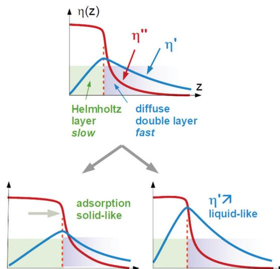
**Fig. 1** Sketch of the solid-like response and the liquid-like response. Adsorption will increase the thickness of the rigid Helmholtz layer. Alternatively, the Newtonian viscosity of the diffuse double layer may increase. Both processes lead to a Sauerbrey-type QCM response.
