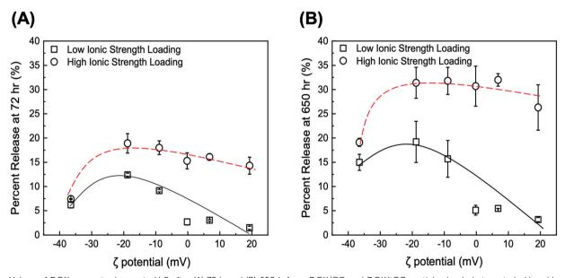
Fig. 6 Values of DOX percent release at pH 5 after (A) 72 h and (B) 650 h from DOX/GO and DOX/tGO particles loaded at neutral pH and low ionic strength (squares) or high ionic strength (circles). Hashed are added to guide the visualization of the results. Error bars represent mean  $\pm$  99% CI ( $n \ge 3$ ).
