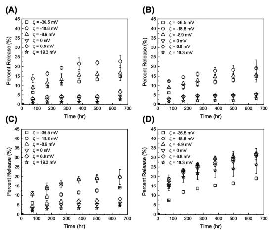
Fig. 5 Release profiles at pH 5 from DOX/tGO particles loaded at (A) pH 4, (B) pH 6, (C) pH 9, and (D) PBS at pH 7.4. Error bars represent mean ± 99% CI (n ≥ 3).
