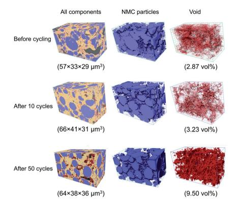
Fig. 3 Reconstructed 3D structures of cathode composite. The figures correspond to the samples before cycling (top), after 10 cycles (middle), and after 50 cycles (bottom). The left column shows all the components (blue: NMC; yellow: LPS; red: void; black: carbon). The middle column shows only the NMC particles, and the right column shows only the voids. The overall volume and void volume percent are labeled below the figures.
