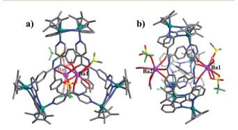
Fig. 8 Molecular structure of trefoil knot 4. Top view (a) and side view (b). Counteranions and hydrogen atoms are omitted for clarity. All hydrogen atoms, anions, and solvent molecules are omitted for clarity except for coordination solvent molecules or anions. Rh teal; Ba pink; N blue; C gray; O red; S yellow; F bright green.
