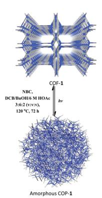
Scheme 1 Recrystallization of COF-1 from the amorphous COP-1 through solvent-assisted linker exchange.
