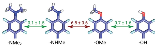
Fig. 7 Average unsigned errors (AUE) for perturbations in the galectin data set using GAFF force field. Values are in \text{kJ mol}^{-1} .
