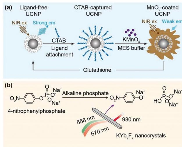
**Fig. 4** Yb-Based UCNPs for biosensing. (a) Schematic design of surface modification and GSH detection by using the  $\alpha$ -NaYbF<sub>4</sub>:Tm (1 mol%)@CaF<sub>2</sub> core-satellite UCNPs. (b) Schematic design for screening the activity of alkaline phosphatase by using the KYb<sub>2</sub>F<sub>7</sub> UCNPs. Reprinted with permission from ref. 30 and 33. Copyright 2018 the Royal Society of Chemistry and 2014 Springer Nature, respectively.
