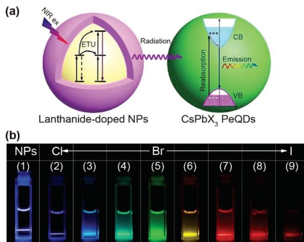
**Fig. 7** Yb-Based UCNP for photoactivation. (a) Schematic representation of the radiative energy transfer upconversion (RETU) processes in PeQDs through sensitization by LiYbF<sub>4</sub>:Tm<sup>3+</sup> (0.5 mol%)/@LiYF<sub>4</sub> core-shell nanoparticles. (b) Photographs of multicolour emission through bandgap tailoring of PeQDs. Reprinted with permission from ref. 112. Copyright 2018 Springer Nature.
