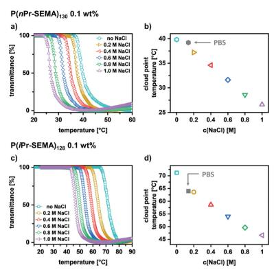
Fig. 5 Influence of the sodium chloride concentration on the cloud point temperature of aqueous (a)  $P(nPr-SEMA)_{130}$  and (c)  $P(iPr-SEMA)_{128}$  solutions (0.1 wt%) showing the common observed "salting-out"-effect for thermo-responsive polymers. A linear dependency of the  $T_{cp}$  values on the salt concentration was observed for both polymers (b and d).
