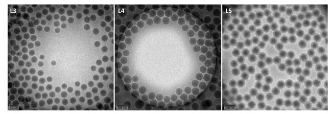
Fig. 1 Cryo-TEM images of P(VAc-co-E) latexes synthesized with 1 wt% macroCTA, at different ethylene pressures: 35 bar (L3), 50 bar (L4) and 100 bar (L5).
