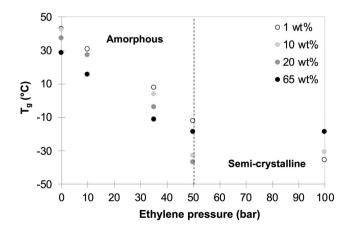
Fig. 3 Variation of  $T_{\rm g}$  as a function of ethylene pressure for different contents of macroCTA (1 to 65 wt% macroCTA/VAc).
