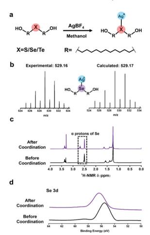
Fig. 1 The characterization of coordination behaviour between chalcogenide containing small molecules and silver tetra fluoroborate. (a) Chemical structure of the coordination compound for (Ag/XC11OH)+. (b) ESI-mass spectrum of (Ag/SeC11OH)<sup>+</sup>. (c) <sup>1</sup>H-NMR (400 MHz, DMSO, 25 °C). (d) XPS results of HOC11Se before and after coordination with silver(ı) cations.
