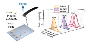
Scheme 1 Quantification of the bond strength between silver(ı) and chalcogenides in sulfur/selenium/tellurium containing block copolymer systems by single-molecule force spectroscopy (SMFS).
