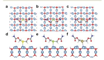
Fig. 5 Top and side views of the optimized geometric structures for  $X(CH_2OCONH_2)_2/Ag_2O$  (200) (a, d) X = S; (b, e) X = Se and (c, f) X = Te. Colors: light blue, Ag; red, O; yellow, S; green, Se; dark yellow, Te; grey, C; blue, N; white, H.
