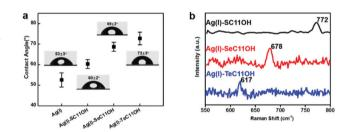
Fig. 3 (a) Static water contact angle of silver only pre-treated and HOC11X modified silver substrates. (b) Raman spectra of SAMs composed of HOC11X formed on silver substrates in the range of  $550-800 \text{ cm}^{-1}$ .
