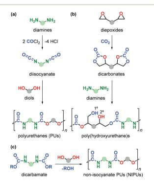
Fig. 22 Synthesis of (a) polyurethanes from diisocyanates and diols, (b) poly-hydroxyurethanes from di(cyclic carbonates) and diamines, and (c) non-isocyanate polyurethanes from dicarbamates and diols. The coloured spheres represent connecting units.
