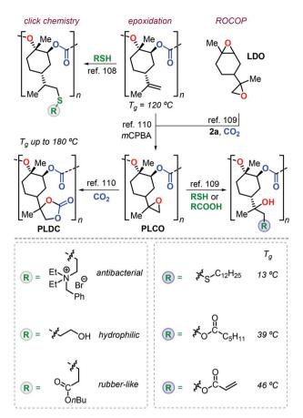
Fig. 7 Functional polymers derived from PLC after post-modification using thiol-ene click reactions or epoxy-based chemistry.
