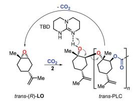
Fig. 8 Depolymerisation mode of PLC promoted by TBD.
