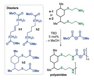
Fig. 26 Synthesis of limonene-based polyamides poly(e-alt-h).
