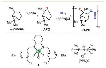
Fig. 3 Synthesis of poly( $\alpha$ -pinene carbonate), PAPC, from  $\alpha$ -pinene, and structures of Cr<sup>III</sup>(salen) complex 1 and [PPN]Cl. mCPBA stands for meta-chloro-perbenzoic acid.
