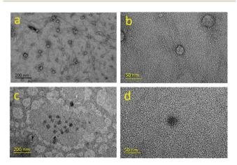
Fig. 5 TEM images for poly(A2-alt-B1)<sub>10</sub> (a, b) and poly(A2-alt-B1)<sub>50</sub> (c, d). 1 wt% samples in deionized water were dried on copper grids for TEM imaging.
