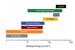
Fig. 2 Summary of binding energies for different interactions. Adapted with permission from ref. 20. Copyright 2017, The Society of Rheology. Adapted from ref. 61 with permission from the Royal Society of Chemistry, copyright 2018.
