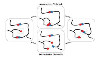
Fig. 1 Representation of associative and dissociative network mechanisms. Adapted with permission from ref. 24. Copyright 2018, American Chemical Society. Adapted from ref. 22 with permission from the Royal Society of Chemistry, copyright 2015.
