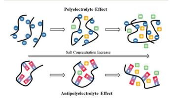
Fig. 11 Schematic representation of polyelectrolyte and antipolyelectrolyte effects. Cationic and anionic moieties are represented in red and blue, respectively, while salt ions are depicted as green and yellow squares.
