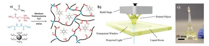
Fig. 20 (a) Chemistry of ionic composite hydrogels via photo-polymerization; (b) fast bottom-up fabrication of high-resolution features from the chemistry above using stereolithography; and (c) 3D printed Eiffel Tower. Adapted with permission from ref. 160. Copyright 2017, John Wiley & Sons, Inc.
