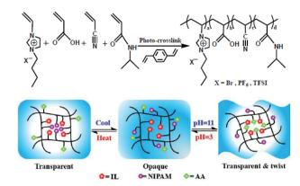
Fig. 10 Reaction scheme for the preparation of PIL-based membranes *via in situ* photo-crosslinking and their mechanism of thermo- and pH-responsive behaviors. Reproduced from ref. 106 with permission from the Royal Society of Chemistry, copyright 2016.
