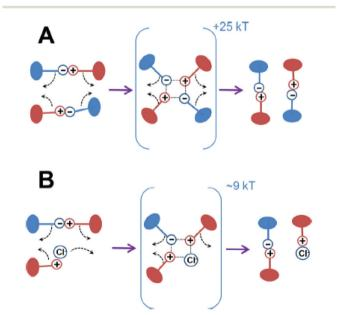
Fig. 6 Rearrangement of ionic interactions (A) in the absence of salt (intrinsic exchange), and (B) in the presence of salt counterions (extrinsic exchanges). Reprinted with permission from ref. 57. Copyright 2019, American Chemical Society.
