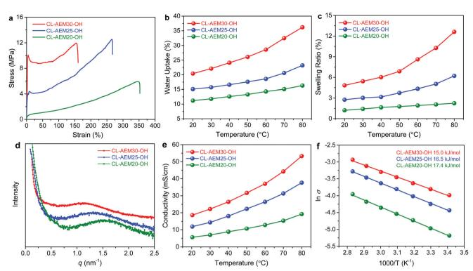
Fig. 1 Crosslinked metallo-polyelectrolyte membranes: (a) stress-strain curves; (b) water uptake; (c) swelling ratios; (d) SAXS profiles; (e) hydroxide conductivity as a function of temperature under fully hydrated conditions; and (f) Arrhenius plots.
