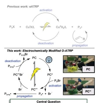
Fig. 1 Previous work demonstrated the ability to mediate ATRP using electrochemistry (top). In this work (bottom), we ask whether this principle can be applied to O-ATRP to control the concentration of PC<sup>-+</sup> and thereby control deactivation in this polymerization method. Figure inset (bottom right) demonstrates the conversion of PC to PC<sup>-+</sup> using potentiostatic bulk electrolysis.
