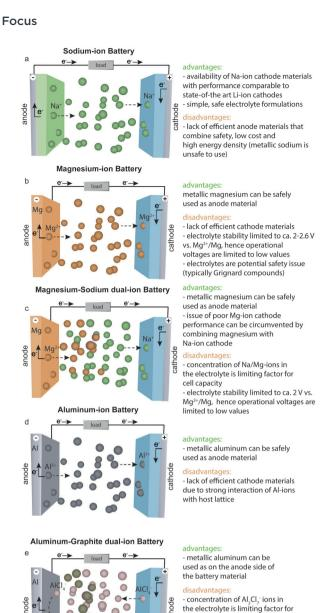
Fig. 3 Schematic working principle of sodium-ion (a), magnesium-ion (b), magnesium-sodium dual-ion (c), aluminum-ion (d), and aluminumgraphite dual-ion (e) batteries and the respective advantages and disadvantages of each system.
