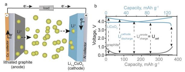
Fig. 1 (a) Schematic illustrating the operating principle of a rechargeable LIB with graphite as the anode material and LiCoO<sub>2</sub> as the cathode material. (b) Galvanostatic charge/discharge curves of LiCoO2 and graphite measured in combination with metallic lithium as counter and reference electrodes (half-cell configuration).
