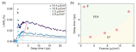
Fig. 4 (a) Time-resolved transient differential reflection spectra of the heterostructure as a function of pump fluence. (b) The appearance time of point  $\beta$  as a function of pump fluence. The area with a yellow background indicates that energy transfer dominates exciton relaxation, while the area with a green background implies that exciton relaxation is dominated by EEA.
