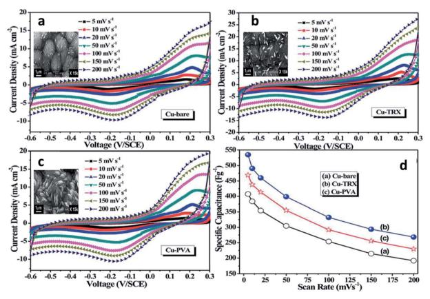
Fig. 16 Cyclic voltammograms of CuO: (a) Cu-bare, (b) Cu-TRX, and (c) Cu-PVA samples at different scan rates. The insets show their corresponding morphologies. (d) Plots of specific capacitance versus potential scan rates for corresponding CuO samples. Adapted from ref. 157 with permission from The Royal Society of Chemistry.
