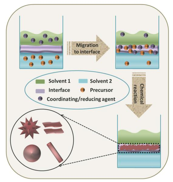
Fig. 11 Schematic diagram of the liquid/liquid interface-assisted synthesis of OD, 1D, 2D or 3D TMOs.
