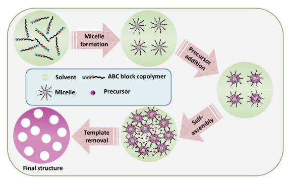
Schematic diagram of the general synthesis strategy of the block copolymer-assisted synthesis of TMOs
