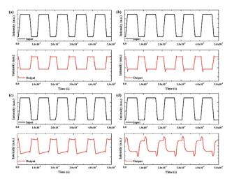
Fig. 6 Temporal response characteristics of an NVCT-based inverter with various square wave input signals of (a) 100  $\mu$ s, (b) 10  $\mu$ s, (c) 100  $\mu$ s and (d) 100  $\mu$ s
