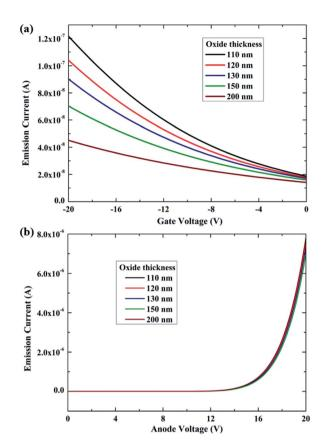
Fig. 4 The (a) transfer characteristic and (b) output characteristic curves of nanoscale vacuum channels with various oxide thicknesses in the linear form
