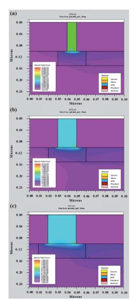
Fig. 2 The electric field intensity distribution of nanoscale vacuum channels with various lengths, (a) 10 nm, (b) 20 nm and (c) 30 nm.
