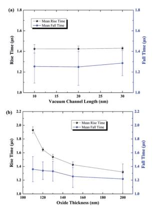
Fig. 7 Simulation results of the temporal response of an NVCT-based inverter with various (a) vacuum channel lengths and (b) oxide thicknesses.
