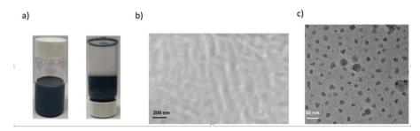
Fig. 5 (a) Photograph of the composite dispersion in a transparent vial after standing for 20 d; (b) cross section SEM image of the fracture surface for the composite coating; and (c) TEM image of the composite dispersion.
