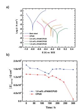
Fig. 6 (a) PDP curves for bare steel, pure CPUD and composite coatings in 3.5 wt% NaCl solution; and (b) plots of  $|Z|_{0.01 \text{ Hz}}$  against the immersion time for pure CPUD and the 1.0 wt% cPANI/CPUD composite coating
