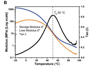
Fig. 1 Thermal Characterisation of ABA (87,60) by DSC (A) and DMTA (B).
