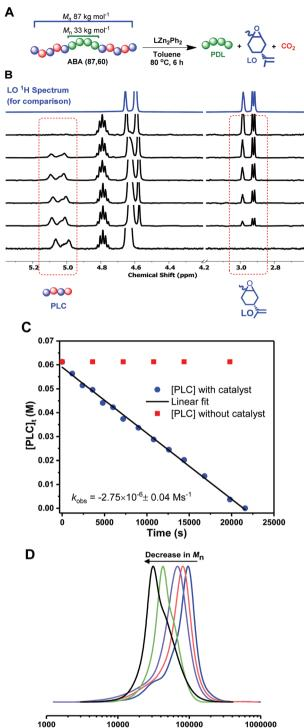
Fig. 4 Deploymerization reactions of ABA (87,60). (A): 1.6 mM of 1; (B) Stacked  $^1$ H NMR spectra (CDCl $_3$ ) taken at various timepoints throughout the depolymerization (LO  $^1$ H NMR spectrum is added for comparison); (C) Kinetic analysis with catalyst 1 (blue circles) and no catalyst (red squares); (D) SEC analysis (THF eluent, vs. PS standards) of aliquots taken at various time-points (see also Fig. S19†).
