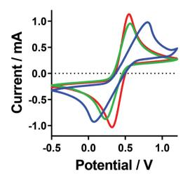
Fig. 7 Cyclic voltammagrams recorded for the [Fe(SO<sub>4</sub>)]<sup>0/+</sup> (blue line),  $[Fe(HSO_4)]^{+/2+}$  (red line) and  $[Fe(SO_4)_2]^{-/2-}$  (green line) systems. All recorded at ambient temperature using an Au working electrode, vs. an Ag/AgCl reference electrode, at 100 mV  $s^{-1}$ . A table of data for the values can be found in the ESI.†
