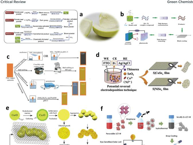
Fig. 12 Some of the most interesting and sustainable approaches to produce green and cost-effective counter-electrodes based on (a and b) waste-derived carbonaceous materials, (c and d) transition metal compounds and (e and f) composite materials. The figures have been adapted from ref. 321, 323, 345, 349, 337 and 358, respectively.
