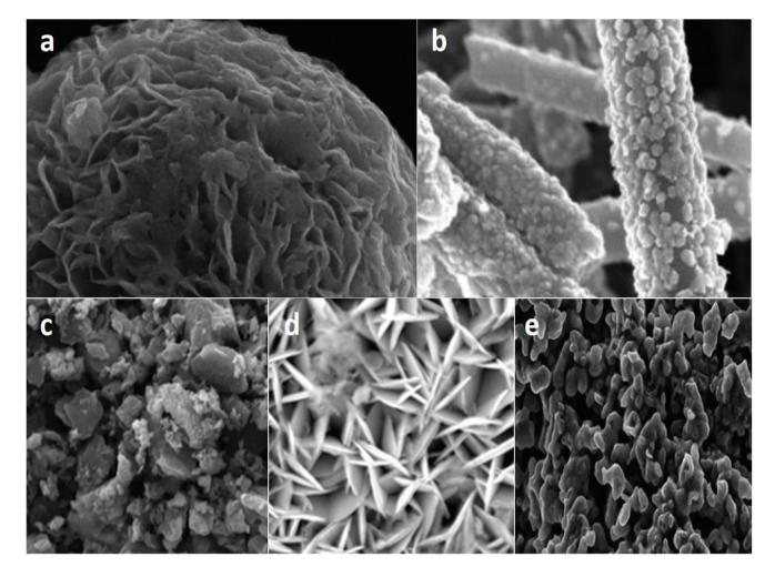
Nanostructures of composite materials: (a) MoS2@rGO nanoflakes (adapted from ref. 355), (b) Ni<sub>3</sub>S<sub>4</sub> nanospheres supported on carbon nanotubes (adapted from ref. 357), (c) graphene-La<sub>2</sub>CdSnTiO<sub>4</sub>-WSe<sub>2</sub> nanopyramids (adapted from ref. 358), (d) hierarchical NiO@NiS@G nanocomposites (adapted from ref. 359) and (e) Ni/CoP<sub>x</sub>@CNTs nanostructures (adapted from ref. 360).
