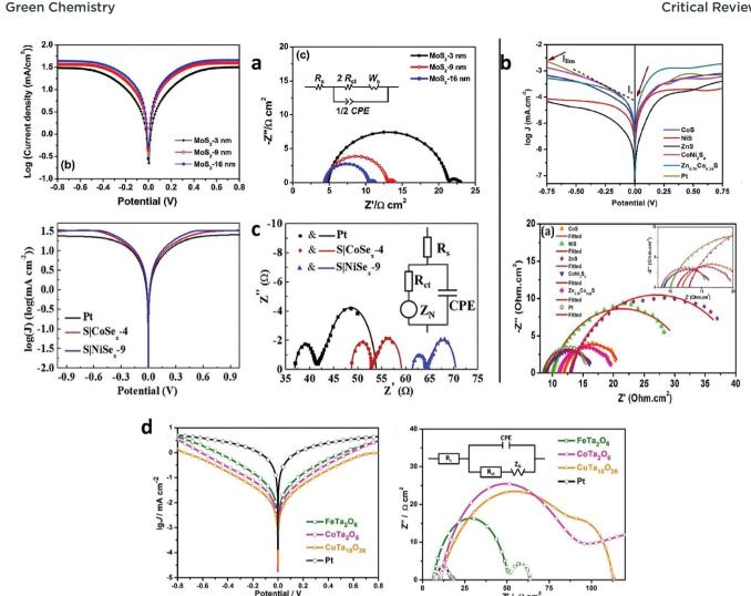
Fig. 10 EIS and Tafel polarization curves of (a) MoS<sub>2</sub> (adapted from ref. 329), (b) different TM sulphides (adapted from ref. 290), (c) cobalt and nickel selenides (adapted from ref. 345) and (d) tantalum-based compounds (adapted from ref. 343).
