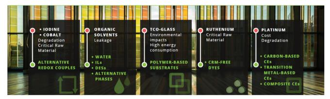
Fig. 3 Main DSSC components, along with corresponding most critical materials, related issues and envisaged solutions.
