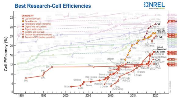
Fig. 2 NREL chart of record performances, showing the highest certified power conversion efficiencies for different types of emerging photovoltaic technologies from 1990 to the present.
