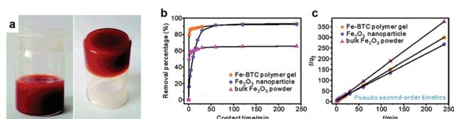
**Fig. 16** (a) Fe(III) BTC (1,3,5-benzenetricarboxylic) CP gel. (b) Percentage of As(v) adsorption with increasing contact time. (c) Pseudo-second-order kinetic plots for As(v) adsorption. Adsorption plots are given for the Fe(III) BTC CP gel, Fe<sub>2</sub>O<sub>3</sub> nanoparticles and bulky Fe<sub>2</sub>O<sub>3</sub> powder at pH 4, 5.0 g L<sup>-1</sup>, 298 K. Reprinted with permission from ref. 161. Copyright 2012 American Chemical Society.
