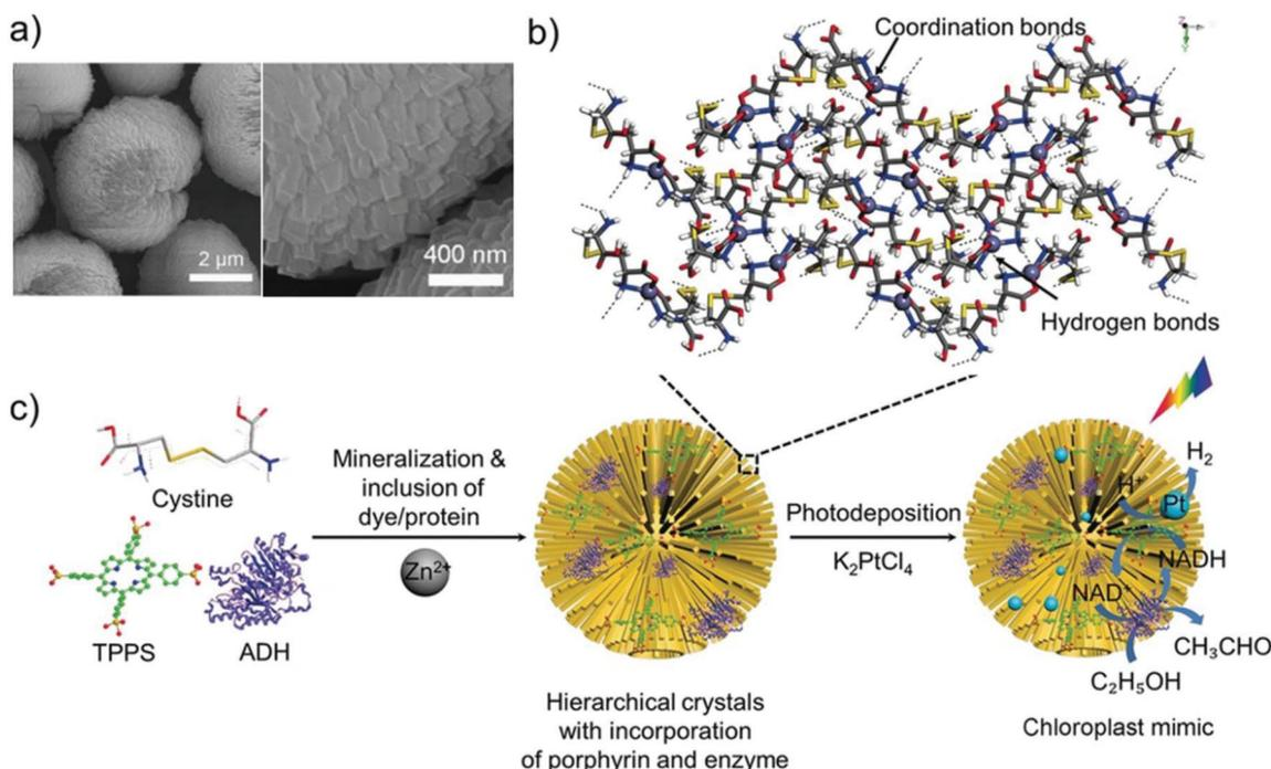
**Fig. 12** Zn(II) cystine CP microspheres: (a) SEM images. (b) Suggested molecular packing based on density functional theory geometry optimisation and crystal structure refinement from powder X-ray diffraction. (c) Schematic representation of the hierarchical chloroplast mimics, prepared by self-assembly of the CP microspheres, followed by encapsulation of porphyrin and enzyme molecules for photoenzymatic reactions. Reprinted from ref. 95 with permission from John Wiley and Sons.
