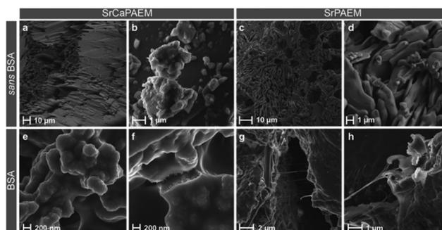
**Fig. 14** SEM images of the Sr<sup>2+</sup>/Ca<sup>2+</sup> CPs SrCaPAEM and SrPAEM pre- (a–d) and post treatment (e–h) with bovine serum albumin. The smoother edges and fibre-like features in e–h are indicative of adsorption of the BSA protein. Reprinted with permission from 129. Copyright (2019) American Chemical Society.
