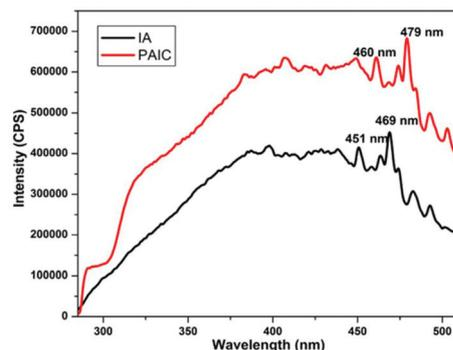
**Fig. 5** Crystals of a luminescent CP based on Ca and itaconic acid, and solid state luminescence spectra of the ligand (IA) and CP (PAIC) at room temperature with  $\lambda_{\text{max}} = 285$  nm. Reprinted from ref. 67 with permission from Elsevier.
