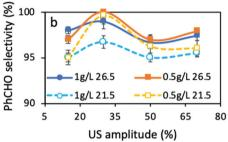
**Fig. 2** The BnOH conversion (a) and PhCHO selectivity (b) after 3 h under four different US amplitudes (15, 30, 50, and 70%), two different catalyst concentrations (0.5 and 1 g  $\rm L^{-1}$ ), and two different temperature of the cooling system (21.5 and 26.5 °C) under irradiation of a solar light simulator (all the experiments were performed more than three times and the standard deviation/error bars were adopted).
