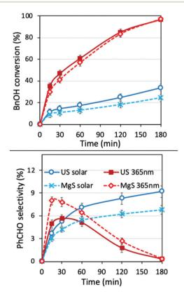
Fig. 7 BnOH conversion (up) and PhCHO selectivity (down) in water as solvent for different light sources (solar: solar light simulator, UV: 365 nm), ultrasound irradiation in pulse mode of 30% amplitude and magnetic stirring (1 g  $\rm L^{-1}$  catalyst, 1 mM BnOH, in acetonitrile at 21.6 °C).
