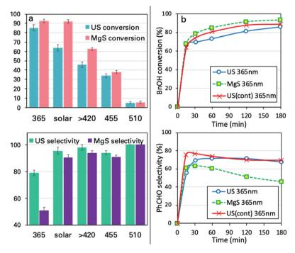
Fig. 5 BnOH conversion (up) and PhCHO selectivity (down) for different light sources after 3 h (a), ultrasound irradiation in pulse mode, continuous mode and magnetic stirring (1 g  $L^{-1}$  catalyst, 1 mM BnOH, in acetonitrile at 21.6 °C) under UV light exposure (b).
