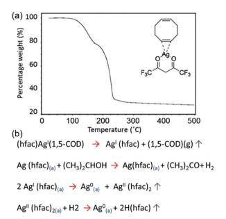
Fig. 19 (a) Thermogravimetric analysis of the decomposition of the pure [(hfac)(1,5-COD)Ag] ink component. (b) The decomposition processes of [(hfac)(1,5-COD)Aq]. Reproduced with permission from ref. 83. Copyright 2016, Rights Managed by Nature Publishing Group.
