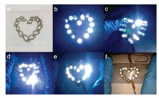
(a) Heart-like circuit drawn by a ballpoint pen; (b) 14 LED lights were lit to show a regular heart shape; LED lights can still work under different deformations; (c) outward bending; (d) inward bending; (e) stretching; and (f) flash photograph under stretching. Reproduced with permission from ref. 136. Copyright 2016, American Chemical Society.
