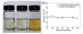
Fig. 15 (a) Optical image of silver citrate particle-free inks: (1) freshly prepared: (2) preserved in the refrigerator for 60 days; (3) preserved under ambient conditions (25 °C) for 60 days; (b) variation of resistivity of printed patterns on a PET substrate cured at 150 °C for 50 min for different storage periods of the ink. Reproduced with permission from ref. 71. Copyright 2012 Flsevier
