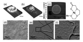
Fig. 10 (a and b) The 3D profilometer image of an inkjet printed, dried and sintered (250 °C, 1 min) droplet of the silver(ı) 2-[2-(2-methoxyethoxy)ethoxylacetate ink; (c) SEM image of a sintered (250 °C, 1 min) droplet; (d-f) SEM images of the printed layer and sintered silver layer (5 min, 250 °C). Reproduced with permission from ref. 82. Copyright 2010, American Chemical Society.
