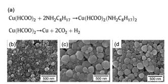
Fig. 21 (a) Chemical reaction in the as-prepared copper formic ink during synthesis and sintering processes; (b–d) SEM images of the copper conductive film obtained by calcination for 60 min at 110  $^{\circ}$ C, 140  $^{\circ}$ C, and 160  $^{\circ}$ C. Reproduced with permission from ref. 52. Copyright 2011 Elsevier.
