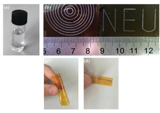
Fig. 17 (a) Optical image of the silver oxalate ink after storage for several months; (b) photographs of the inkjet printing patterns cured at 150 °C for 30 min; (c) image of the bent patterns and (d) picture of tape test for the inkjet printing line. Reproduced with permission from ref. 51. Copyright 2015 Elsevier.
