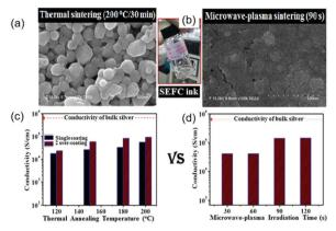
Fig. 8 Comparison of the effects of thermal annealing (left) and microwaveplasma sintering (right) on the surface morphology and conductivity of the films deposited on glass with a SEFC-based ink. Reproduced with permission from ref. 130. Copyright 2016 Elsevier.
