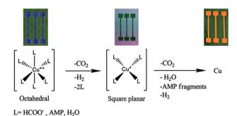
Fig. 23 A suggested mechanism for the decomposition of the complex from an octahedral to a square planar configuration to metallic copper. An image of the obtained film at each stage is presented on top. Reproduced with permission from ref. 101. Copyright 2015, Royal Society of Chemistry.
