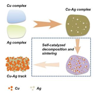
Fig. 25 Schematic illustration of self-catalyzed decomposition and sintering of Cu-Ag complex inks. Reproduced with permission from ref. 134. Copyright 2018, Royal Society of Chemistry.
