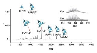
Fig. 2 Positive ESI-MS spectrum of  $Im^5{}_3Bz$  (normalized by its most intense fragment at m/z=564.3 from the free ligand) in acetonitrile (2.0  $\times$  10<sup>-3</sup> M) in the presence of  $Zn^{2+}$  (1.6  $\times$  10<sup>-3</sup> M). Inset: isotopically resolved signals at m/z=965.3 and the calculated isotopic distributions for  $[(Im^5{}_3Bz)_4(Zn^{2+})_3(OSO_2CF_3)_3]^{3+}$ . Objects correspond to the mass peak assignment (L:  $Im^5{}_3Bz$ , M:  $Zn^{2+}$ , T:  $OSO_2CF_3^{-}$ ).
