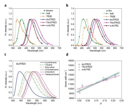
Fig. 3 Steady-state photophysical properties of the TSCT-HABs. PL spectra of the TSCT-HABs in toluene ( $10^{-5}$  mol L<sup>-1</sup>) (a) and in the film state (b), PL spectra of Ac3TRZ3 in solvents with different polarity (c), and the linear correlation of orientation polarization ( $\Delta f$ ) of the solvent with the Stokes shift for the TSCT-HABs (d) (see Table S1† for data).
