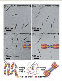
Fig. 3 Self-seeding behaviour of PFS $_{26}$ -b-PNIPAM $_{520}$  and PFS $_{35}$ -b-P2VP $_{400}$  fragment mixtures (mass ratio 1 : 1). (a–d) TEM images of the micelles obtained by annealing the mixture for 30 min at (a and c) 80 °C, and (b and d) 90 °C. (a) and (b) show the comicelles before staining, while (c) and (d) show the comicelles after selectively staining the P2VP block with PtNPs. (e) Schematic diagram of the self-seeding process of the mixture.
