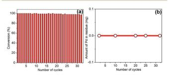
Fig. 8 (a) Reusability potential of the catalyst for quinoline hydrogenation in water using THDB reductant. (b) ICP-OES data showing the evidence of no leaching of Pd from the dip-catalyst after a large number of cycles.
