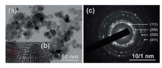
Fig. 5 (a) TEM image of Pd nanoparticles anchored on the surface (b) HRTEM image and (c) SAED of Pd@GS.
