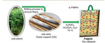
Fig. 2 Schematic illustration for the synthesis of Pd@GS.
