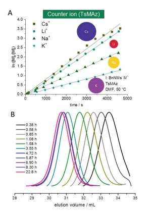
**Fig. 4** (A) Kinetic plots of  $\ln([M]_0/[M]_t)$  vs. time for the azaanionic polymerization of TsMAz with BnNHMs (initiator) in DMF-d<sub>7</sub> at 50 °C with different bis(trimethlsilyl)amide-salts. (B) SEC-kinetics of MsMAz, BnNKMs at 50 °C in DMF (RI-signal), reproduced from ref. 143 with permission from Royal Chemical Society, copyright 2017.
