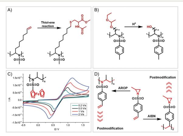
Fig. 6 Functional polyaziridines: (A) terminal double bond can be converted *via* thiol—ene reaction. (B). Acetal-protected polyaziridines yield hydroxyl functionalities. (C) Ferrocene-containing polyaziridines are redox-responsive. (D) Orthogonal aziridine allows anionic and radical polymerization.
