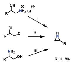
Scheme 3 Synthesis of aziridines with and without a ring substituent (R) by i: the β-chloroethylamine process, ii: the Dow Process, iii: the Wenker synthesis.
