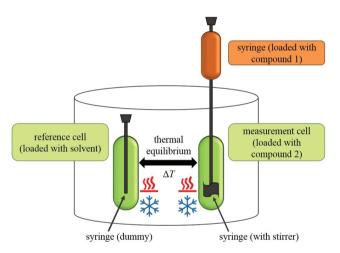
Fig. 2 General setup of an ITC instrument.
