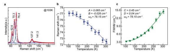
Fig. 4 Temperature-dependent Raman spectra of the CsPbBr<sub>3</sub> microspheres. (a) Raman spectrum of the CsPbBr<sub>3</sub> microspheres measured with a 633 nm excitation laser at 103 K. Five Raman peaks at 62.6, 70.3, 76.4, 127.2 and 126 cm<sup>-1</sup> are obtained by peak fitting. (b) and (c) Temperature dependence of position and line width of the Raman mode at 76 cm<sup>-1</sup>. Inside are fitting parameters using the equations from ref. 54.
