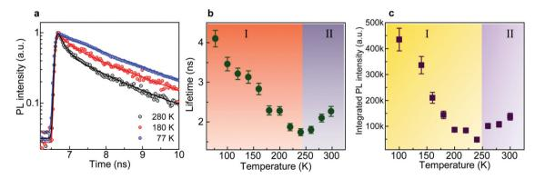
Fig. 5 Time-resolved PL (TRPL) of  $CsPbBr_3$  microspheres. (a) TRPL decay curves of  $CsPbBr_3$  microspheres with different temperatures monitored around 530 nm with excitation of 400 nm (76 MHz, 120 fs). (b) The PL lifetime of  $CsPbBr_3$  microspheres decreases with temperature from 77 K to 238 K, while it increases with temperature from 238 K to 300 K. (c) Plot of the change in integrated PL intensity with temperature from 77 K to 300 K. It almost shares the same feature as shown in (b).
