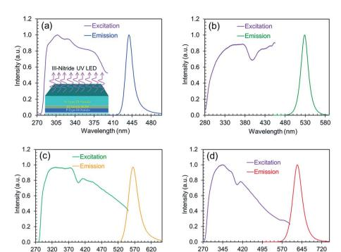
Fig. 5 The normalized excitation spectra along with the corresponding normalized emission (blue, green, yellow, and red) spectra.
