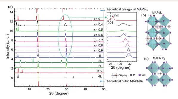
Fig. 1 (a) The XRD spectra of MAPbBr<sub>3</sub> with varying ligand concentration and MAPb(Br<sub>x</sub> $l_{1-x}$ )<sub>3</sub> with varying 'Br': 'I' ratio. (b) The primitive cell of cubic-structured MAPbBr<sub>3</sub>. (c) The primitive cell of tetragonal-structured MAPbI<sub>3</sub>.  $L=15~\mu L$  of ligand (octylamine).
