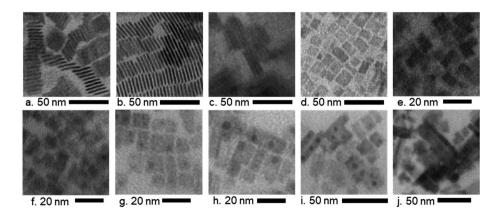
Fig. 2 TEM images of (a-e) MAPbBr<sub>3</sub> with decreasing ligand concentration (4L, 3.5L, 2L, and 1L) and (f-j) MAPb(Br<sub>x</sub>l<sub>1-x</sub>)<sub>3</sub> with increasing iodine content (x = 0.8, x = 0.6, x = 0.5, x = 0.4, and x = 0) and fixed ligands (1L).
