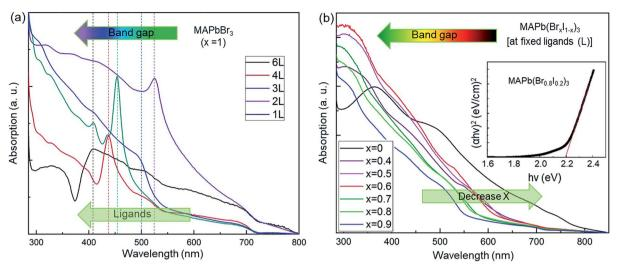
Fig. 3 Optical absorption spectra of (a) MAPbBr<sub>3</sub> with ligand concentration variation and (b) MAPb(Br<sub>x</sub>l<sub>1-x</sub>)<sub>3</sub> with 'Br' and 'I' composition variation at a fixed ligand amount (1L), and inset is the Tauc plot of the sample at x = 0.8.
