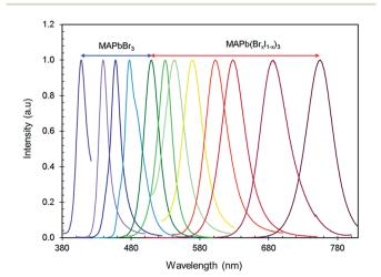
Fig. 4 The normalized PL emission spectra of halide perovskite nanocrystals over the range of 408-755 nm with varying ligand concentration for MAPbBr<sub>3</sub> and composition of 'Br' and 'I' for MAPb(Br<sub>x</sub>I<sub>1-x</sub>)<sub>3</sub>.
