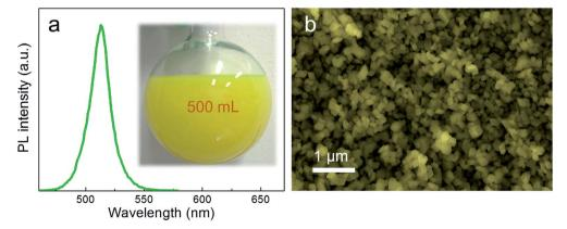
Fig. 4 (a) PL spectrum of large-yield CsPbBr<sub>3</sub>@Cs<sub>4</sub>PbBr<sub>6</sub> NCs, inset is the photograph of large-yield reaction product. (b) Large-scale SEM image of high yields of CsPbBr<sub>3</sub>@Cs<sub>4</sub>PbBr<sub>6</sub> NCs.
