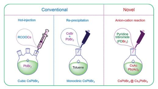
Fig. 2 Schematic of the hot-injection, re-precipitation and anion-cation reactions for cubic CsPbBr<sub>3</sub>, monoclinic CsPbBr<sub>3</sub> and CsPbBr<sub>3</sub>@-Cs<sub>4</sub>PbBr<sub>6</sub> NCs.
