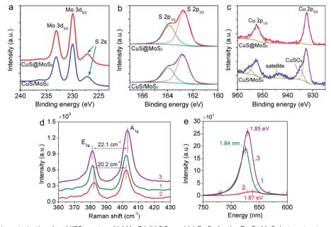
Fig. 2 Spectroscopic characterization. (a-c) XPS spectra of (a) Mo 3d, (b) S 2p and (c) Cu 2p for the Cu<sub>x</sub>S@MoS<sub>2</sub> heterostructures and conventional MoS<sub>2</sub> monolayer transferred onto Cu<sub>x</sub>S nanocrystals. (d) Raman and (e) photoluminescence spectra of (1) monolayer MoS<sub>2</sub> inside the dotted lines in Fig. 1c, (2) conventional MoS<sub>2</sub> monolayer transferred onto Cu<sub>x</sub>S nanocrystals and (3) Cu<sub>x</sub>S@MoS<sub>2</sub> heterostructures
