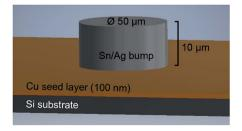
Fig. 1 Schematics of the investigated Sn/Ag solder bumps. A layer of 10 μm Sn/Ag is electrochemically deposited on a Cu coupon. The Ti and Ti<sub>x</sub>/SiO<sub>2</sub> layers are not shown to simplify the image.
