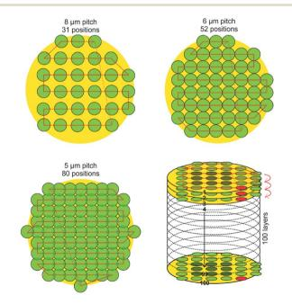
Fig. 2 Schematics of three different grid layouts that are generated and placed over the target using the in-house written software suite. The decrease of the pitch size from 8  $\mu$ m to 5  $\mu$ m allows scanning the targeted area by 80 surface positions in comparison to 31 positions, respectively. At the bottom right, a schematic of the complete measurement protocol to measure multiple sample layers is illustrated, with the starting grid position highlighted in red.
