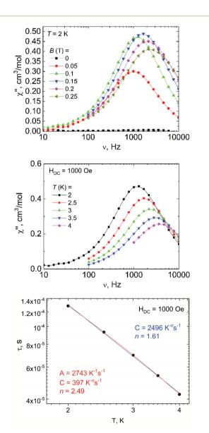
Fig. 8 AC susceptibility data for 2b. The out-of-phase susceptibility  $\chi'$ at various static magnetic fields (above) and as a function of temperature measured at  $B_{DC}$  = 0.1 T (middle). The analysis of the relaxation times derived from the AC susceptibility data for 2b with the Raman relaxation process (blue line) or with a combination of direct and Raman processes (red line) (below).
