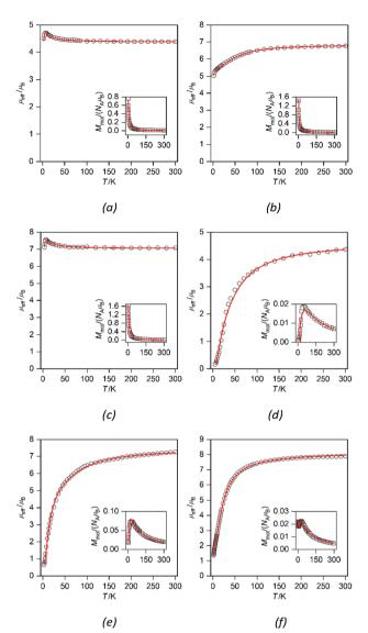
Fig. 7 Magnetic data for 2a (a), 2b (b), 2c (c), 4a (d), 4b (e) and 4c (f) depicted as temperature dependence of the magnetic moment calculated from the molar magnetization measured at B = 0.5 T shown in the inset. Experimental data are shown as empty circles, and fitted data are shown as red lines.
