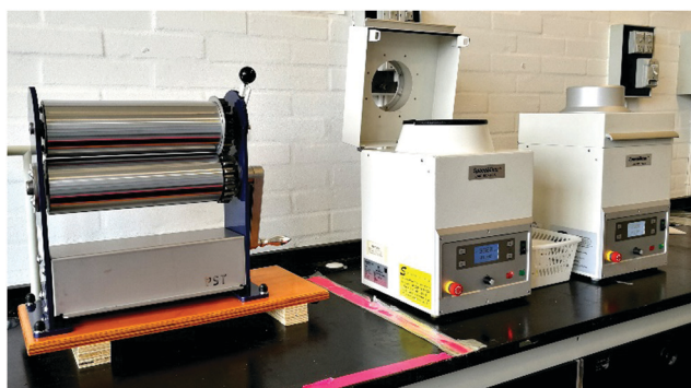
Fig. 9 Laboratory-scale mixers. From the left: roll mill with two rolls and two speed mixers. Optimised mixing is required for reliable elastomers, and for most silicone elastomer formulations high shear mixing is strictly required.
