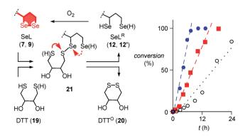
Fig. 4 Oxidation of 500  $\mu$ M 19 to 20 as a function of time in the absence ( $\bigcirc$ ) and the presence of 500  $\mu$ M 9 ( $\blacksquare$ ) and 22 ( $\bullet$ ) in D<sub>2</sub>O, pD = 8.0, with linear fits to determine the  $t_{50}$ . Structures are shown in neutral form, acidic protons are indicated in parenthesis. Competing ring closures in reactive intermediate 21 are indicated with solid (preferred) and dashed red arrows.
