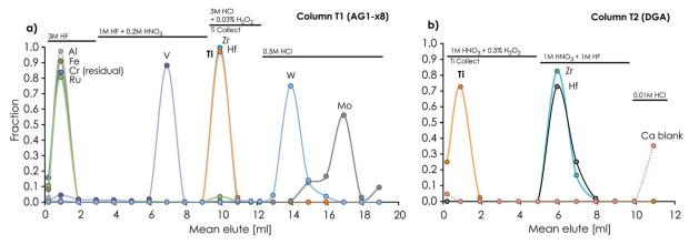
Fig. 4 Ion chromatographic elution profiles of elements separated on (a) the anion exchanger (600  $\mu$ l AG1-x8 200–400 mesh) column T1 (ID = 3.5 mm, L = 62 mm), which separates Ti (together with Zr and Hf) from Al, Fe, Ru, V, W and Mo, and (b) the 3<sup>rd</sup> Ti purification column (T2, ID = 3.5 mm, L = 27 mm) packed with 250  $\mu$ l of DGA-N 50–100  $\mu$ m resin.
