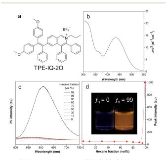
Fig. 2 (a) Molecular structure of TPE-IQ-2O. (b) UV-vis spectrum of TPE-IQ-2O in DMSO. (c) Photoluminescence (PL) spectra of TPE-IQ-2O in THF/hexane mixtures with different hexane fractions ( $f_{\rm H}$ ). (d) Plot of relative PL intensity ( $I/I_0$ ) versus  $f_{\rm H}$ . Inset: fluorescent photos of THF/hexane mixtures of TPE-IQ-2O at  $f_{\rm H}=0$  and 99 vol% taken under 365 nm UV illumination from a hand-held UV lamp. Concentration: 10  $\mu$ M;  $\lambda_{\rm ex}$ : 430 nm.
