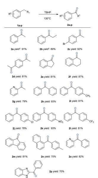
Scheme 1 Substrate scope. <sup>ab a</sup> Alkylarene or diarylmethane (1 mmol), TBHP (hexane solution, 2 ml,  $\sim$ 12 equiv.), 130 °C in pressure tube. <sup>b</sup> Isolated yields. <sup>c</sup> GC yields.
