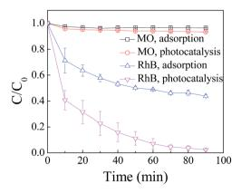
Fig. 1 Degradation of RhB and MO by adsorption and photocatalysis. The concentration of RhB and MO was 15 mg  ${\rm L}^{-1}$  and the dosage of  $Znln_2S_4$  was 0.1 g L<sup>-1</sup>.
