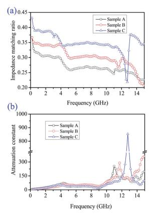
Fig. 10 Frequency-dependence of (a) impedance matching ratio ( $Z_r$ ) and (b) attenuation constant ( $\alpha$ ) of different Ni/ZnO composites.
