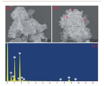
Fig. 4 (a and b) SEM images and (c) EDS pattern of the Ni/ZnO composites prepared in the solvent solution containing 30 mL distilled water and 30 mL glycerol.
