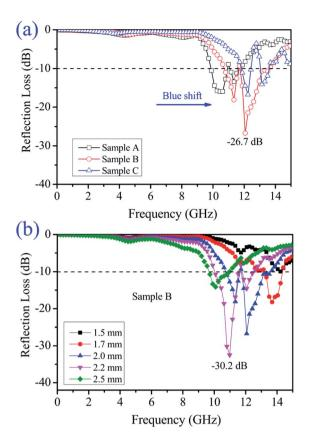
Fig. 9 (a) Reflection loss (RL) of the different Ni/ZnO composites with a thickness of 2.0 mm and (b) RL of the core—shell Ni@ZnO (Sample B) composite with various thicknesses.
