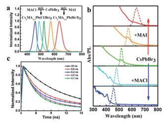
Fig. 5 (a) An overview of the PL spectra of the samples obtained by mixing CsPbBr<sub>3</sub> NCs with either MACl or MAI NCs in various ratios (λ<sub>ex</sub> = 365 nm for all). (b) Evolution of the optical absorption (solid lines) and PL (dashed lines) spectra of CsPbBr3 NCs with the increasing quantities of MAX (X = Cl and I), added as ion-exchange sources. (c) Evolution of the time-resolved PL decay spectra of CsPbBr3 NCs and mixing with either MACI or MAI NCs at various ratios.
