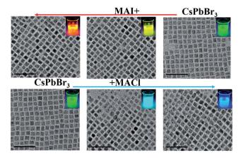
Fig. 4 TEM images of the CsPbBr<sub>3</sub> NCs after treatment with various quantities of MAI (up) and MACI (down). The insets show the evolution of emission colors (under a UV lamp,  $\lambda_{\text{ex}} = 365 \text{ nm})$  from crude CsPbBr<sub>3</sub> NCs to composited perovskite NCs. Scale bars correspond to
