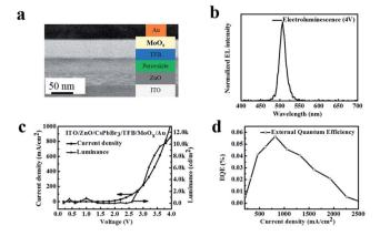
Fig. 7 (a) Device structure of the CsPbBr<sub>3</sub> perovskite LEDs. Schematic and the cross-sectional TEM image of the device: ITO/ZnO/perovskite/TFB/MoO<sub>x</sub>/Au. (b) Normalized EL spectrum of the CsPbBr<sub>3</sub> perovskite thin film-based LEDs at the applied voltage of 4 V. (c) Current density and luminance for the CsPbBr<sub>3</sub> perovskite LED measured at room temperature. (d) The external quantum efficiency (EQE) versus current density curves of this LED.
