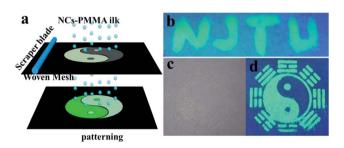
Fig. 6 (a) The schematic of patterning by screen printing. (b), (d) Images ( $\lambda_{ex} = 365$  nm) and (c) (under daylight) of the patterning obtained using the mixture of CsPbBr<sub>3</sub> NC-PMMA.
