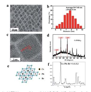
Fig. 2 (a) TEM image of the colloidal CsPbBr $_3$  NCs. (b) Size distribution analysis for the sample. (c) High-resolution TEM image of the colloidal CsPbBr $_3$  NCs. (d) XRD patterns of the colloidal CsPbBr $_3$  NCs. (e) Molecular structure model, and (f) EDX spectrum of the colloidal CsPbBr $_3$  NCs.
