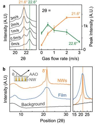
Fig. 2 (a) (left) XRD patterns of nanowire-filled templates crystallised at various assisted gas-flow rates. (right) Based on the normalised XRD patterns, the average intensity of the peak at 21.6° and 22.6° is plotted as a function of assisted-gas flow rate. (b) XRD patterns of a nanowire-filled template (orange), melt-quenched film (blue), and silicon background (grey). The right image shows the magnification of the  $\delta'$ -phase range.
