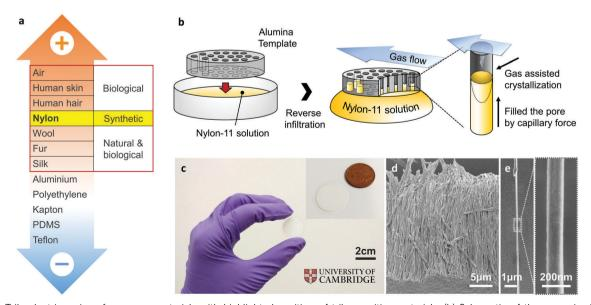
Fig. 1 (a) Triboelectric series of common materials with highlighted position of tribo-positive materials. (b) Schematic of the nanowire fabrication procedure. (c) Photographs of a fabricated nanowire-filled AAO template. The inset shows size comparison with a British one-pence coin. (d and e) SEM images of template-freed nanowires and a single strand of Nylon nanowire, respectively
