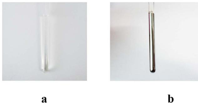
Fig. 6 Photos of  $2^{2+} \cdot 2PF_6^-$  ( $4.5 \text{ mM L}^{-1}$ ) taken 10 min (a) and 10 h (b) after treatment with 4 molar equiv. of  $AgNO_3$  in a mixture of  $CD_3CN$ ,  $D_2O$ , and  $ND_3 \cdot D_2O$  (25–28% by mass) (1/0.4/0.007, v/v/v) at 323 K.
