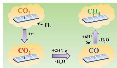
**Fig. 9** The possible pathway for electrochemical reduction of CO<sub>2</sub> to CH<sub>4</sub> on Zn-MOF/CP cathode in ILs.
