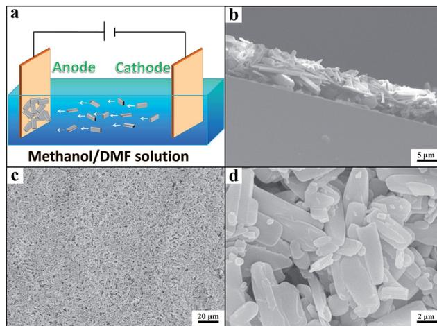
Fig. 2 The schematic diagram of fabrication procedure and SEM images of Zn-MOF/CP cathode using the Zn-MOF synthesized at  $x = 0.38$ . (a) Schematic diagram of fabrication procedure. (b) SEM image to show the thickness Zn-MOF on the CP. (c) SEM image of the surface. (d) Amplified SEM image of the surface.
