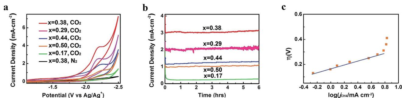
Fig. 4  $\text{CO}_2$  reduction performance of Zn-MOF/CP cathodes. (a) CV traces. (b) Current density profiles. (c) Tafel plot for  $\text{CH}_4$  of the Zn-MOF/CP cathode using Zn-MOF synthesized at  $x = 0.38$ .
