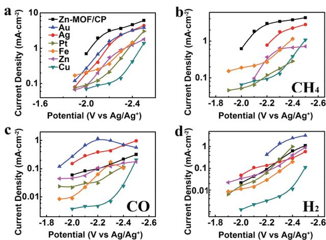
**Fig. 7** Current densities obtained from the Zn-MOF/CP cathode prepared using Zn-MOF synthesized at  $x = 0.38$  and various metal cathodes. (a) Total current densities. (b) Partial current densities of CH<sub>4</sub>. (c) Partial current densities of CO. (d) Partial current densities of H<sub>2</sub>.
